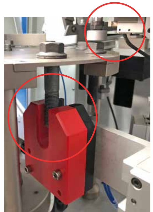
Fig. 1 – ibg fork coil for microstructure testing and ibg crack test probe at work
